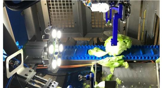
Series 3 of the CoreTakt lettuce corer has launched commercially following extensive testing
