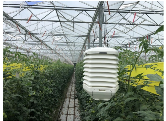
Autogrow's wireless smart sensor, Foliium
