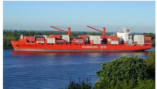
Ship offers a container storage capacity of 3,800 TEU and is equipped with 1,000 reefer plugs
