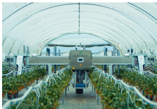
Each of the robot's arms can pick one strawberry every five seconds
