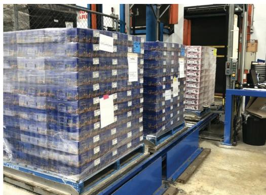
Palletised products travel over a conveyor belt to be treated p.p1 {margin: 0.0px 0.0px 0.0px 0.0px; line-height: 11.1px; font: 7.0px Adelle}
